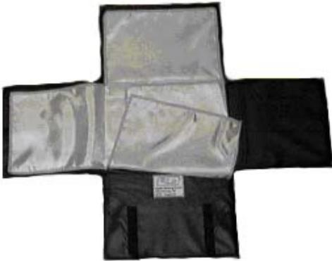
Manufactured from TWARON™ the function of this bag is to prevent damage from fragments caused by an exploding letter bomb. The bag will carry an envelope up to DIN A4 size and approximately 40 mm thick. A special exchangeable cloth, vacuum metallized on both sides, gives additional protection against radio interferences. In tests and incidents it was proven that all fragments caused by the explosion were captured inside the bag and could be handed over to the forensic laboratory for analysis.
